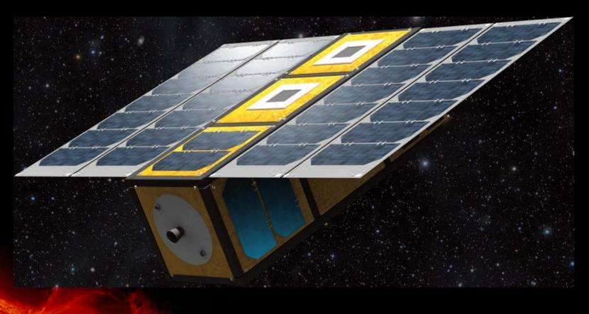
\* Shown with DSI COMET-1 Water Thruster Integrated. Flight articles used will incorporate Reflectarray Rectennas (combination solar/receive & transmit antennas).
