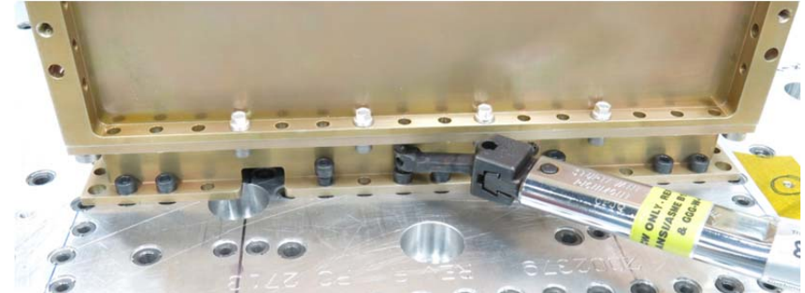
Figure 25: Using Reduced Clicker Head to Torque Fasteners
