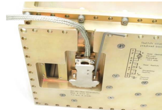
Figure 26: Installing CSD Initiator Electrical Harness
