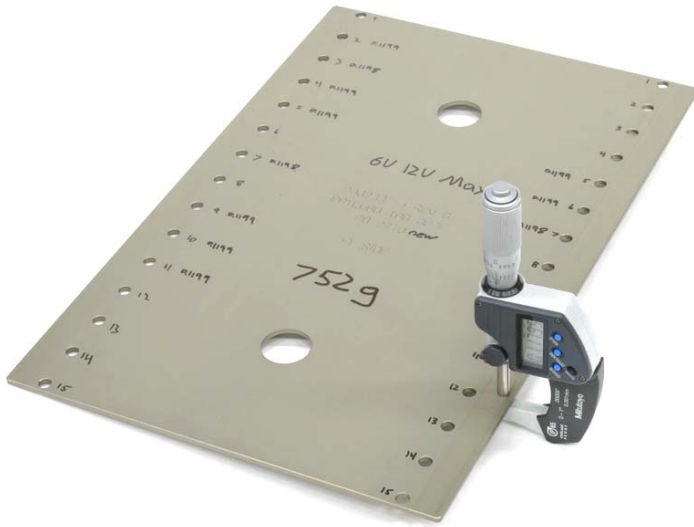
Figure 14: Measuring Tab Thickness with Micrometer
