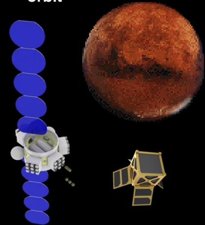
The CubeSat carrier or ESPA OMS using high efficiency propulsion can carry up to 27 – 3U CubeSats to Mars.
