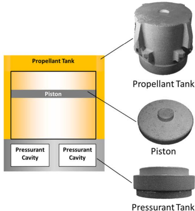
Figure 7: As-Printed EBM Additive Manufactured Piston Tank Components
