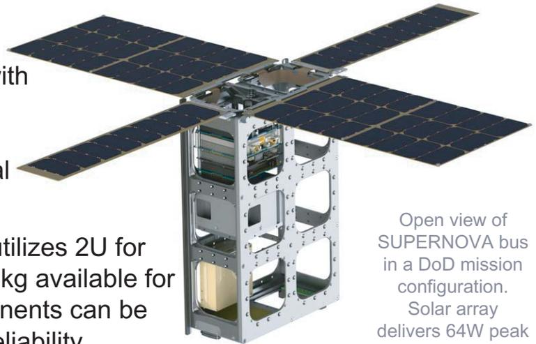
Open view of SUPERNOVA bus in a DoD mission configuration. Solar array delivers 64W peak
