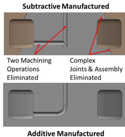
Figure 4: Internal Passages Enable Elimination of Processes
