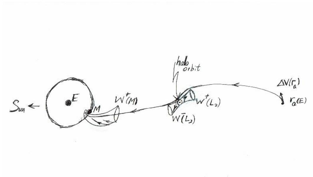
Figure 2. Trajectory from  $r_a(E)$ , passing near the stable manifold ( $W^+$ ) and unstable manifold ( $W^-$ ) of  $L_2$ . These manifolds exist in position-velocity space and are shown here projected into position space, as an illustration. The trajectory is then guided to the Moon via another stable manifold,  $W^+$ , of the lunar WSB where lunar capture occurs for  $0 \Delta V$ . (Earth-Sun rotating coordinates)
