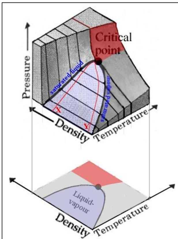
The liquid-vapour area describes what's happening in your tanks: a subcritical region where both the liquid and vapour phases coexist.
