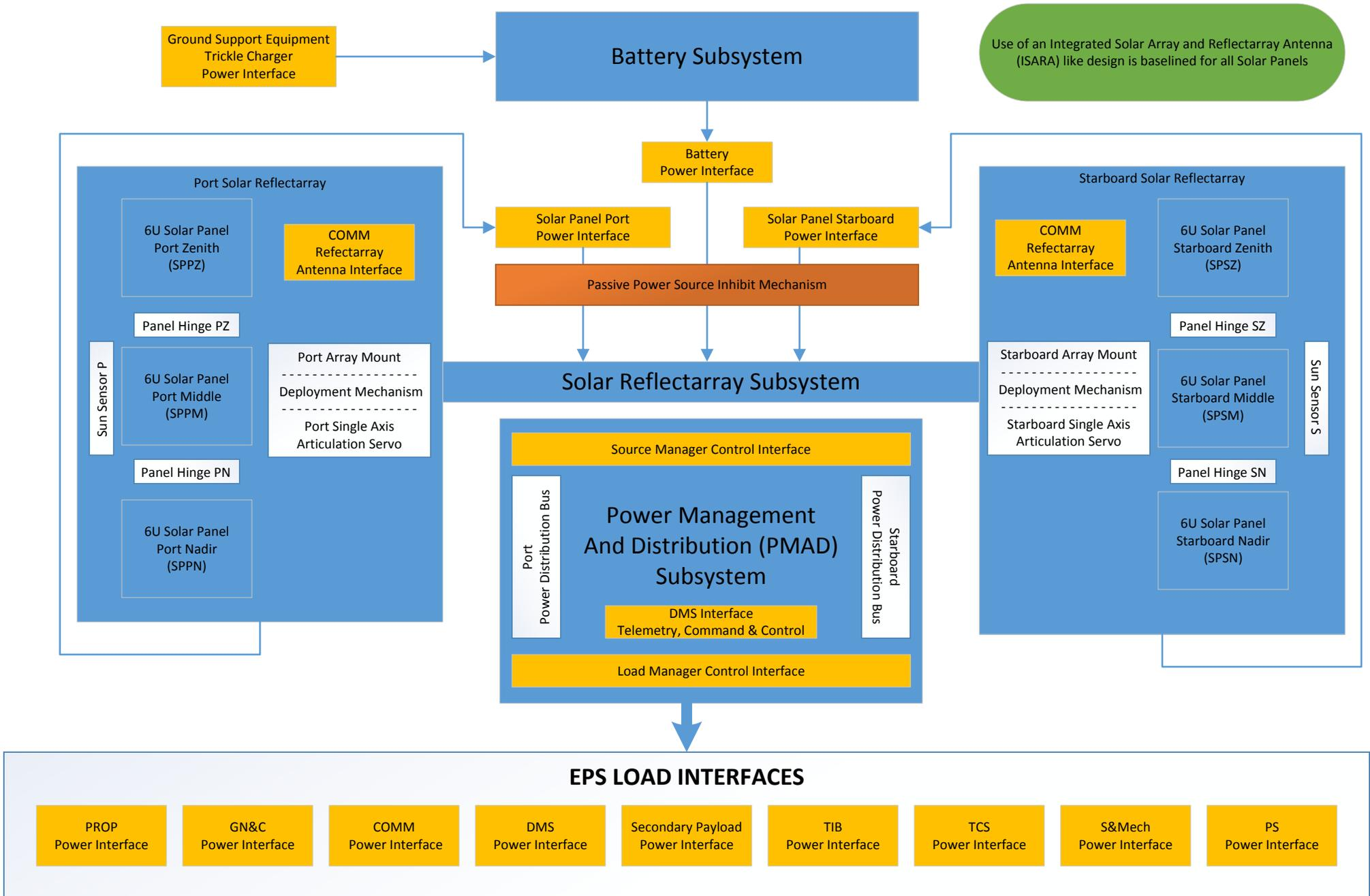
Use of an Integrated Solar Array and Reflectarray Antenna (ISARA) like design is baselined for all Solar Panels
