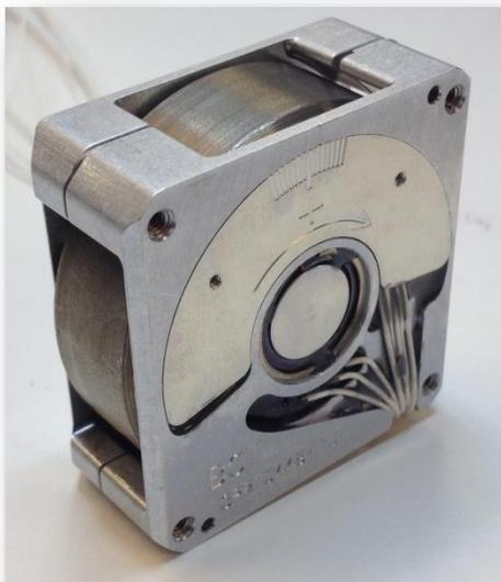
The BCT Micro Reaction Wheel uses a BCT-built motor and a long life hybrid bearing and lubrication system. The wheels undergo extensive testing to characterize their electrical and mechanical performance, including jitter and life test.
