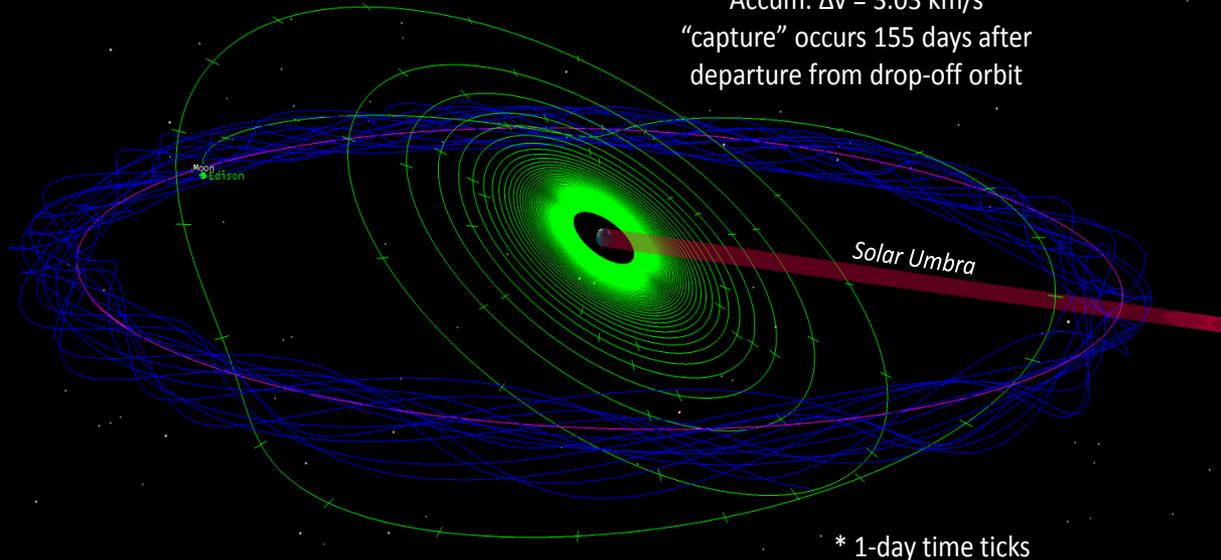
Lunar Cube trajectory from MEO to lunar intercept (green trace) and lunar capture/orbit (blue trace). ( $\approx 8\text{kg}$  s/c wet mass) Courtesy of JPL.
