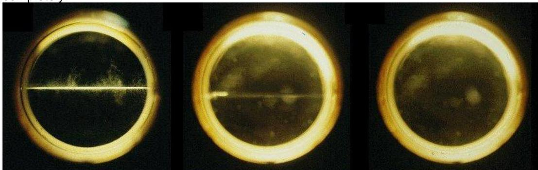
Supercritical nitrous can therefore be regarded as either a super-dense gas, or a low density liquid.
