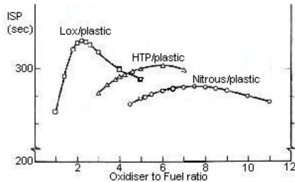
So you'll still get plenty of thrust even if your mixture ratio of nitrous to fuel is way off 7:1, which is good if your test rig can't give you accurate figures to let you tune up the motor: the first few flights will still be adequate, provided the motor doesn't melt.
