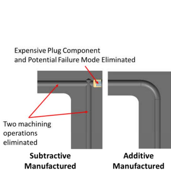
Figure 3: Internal Passages Enable Elimination of Components
