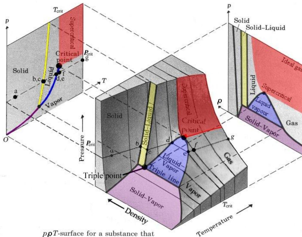
$ppT$ -surface for a substance that expands on melting. Projections of the surface on the  $pT$ - and  $pp$ -planes are also shown.
