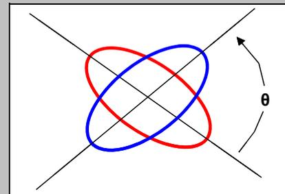
Polarization Angle ( $\theta$ )  $\equiv$  Angle between transmit and receive major axes.
