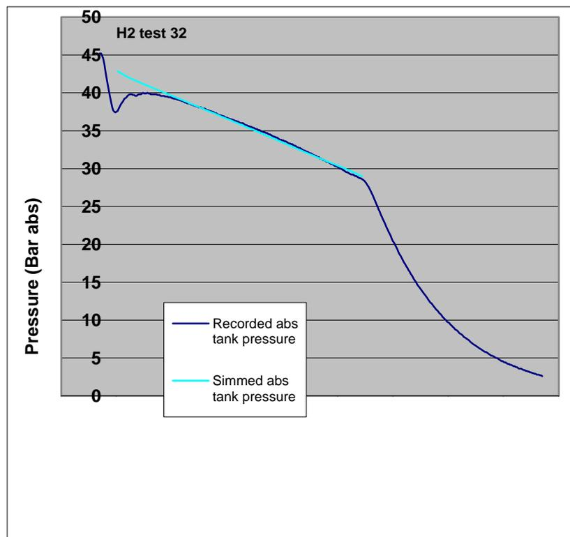
The lower the pressure drops below vapour-pressure, the more vapour is required to raise the pressure back up, and the more chilled the liquid-phase becomes as it provides this vapour. This is why leaks in any pipe-joints carrying the liquid phase of nitrous oxide show up as regions covered in ice; the nitrous sucks heat out of the atmosphere as it leaks out to atmospheric pressure and vaporises, freezing the water-vapour in the air around the leak.
