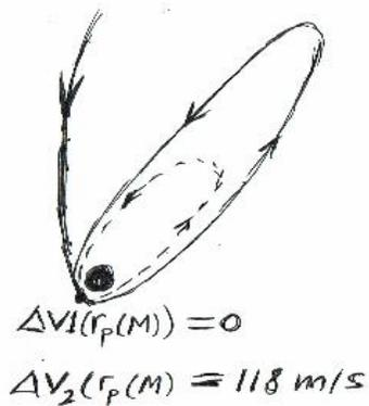
Figure 3. Arrival of trajectory into ballistic capture at  $r_p(M)$  so that  $\Delta V_1(r_p(M)) = 0$ . The initial osculating elliptical orbit has  $r_a(M) = 40,000 \text{ km}$ . A maneuver of  $\Delta V_2 = 118 \text{ m/s}$  reduces  $r_a$  to  $r_a(M) = 10,000 \text{ km}$  (dashed ellipse).
