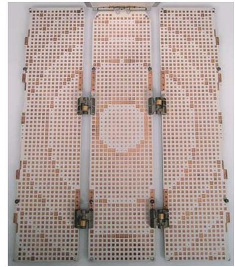
Reflectarray side of three-panel depolyable PMDSAS array
