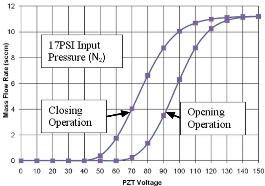
Hysteresis is inherent to the piezo actuator and is repeatable. Mass flow rate is calculated as a function of valve excitation and valve direction.
