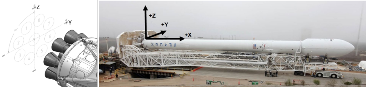
Figure 4-1: Launch Vehicle Coordinate Frame
