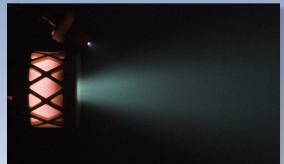
BIT-1 Operating with Xenon at 13W
